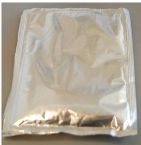
Typical Packaging Material: Aluminium PE multi-laminar bags
