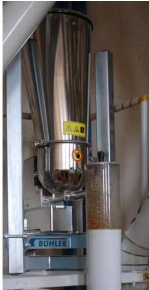
Typical Microfeeder dosing wheatflour with premix
